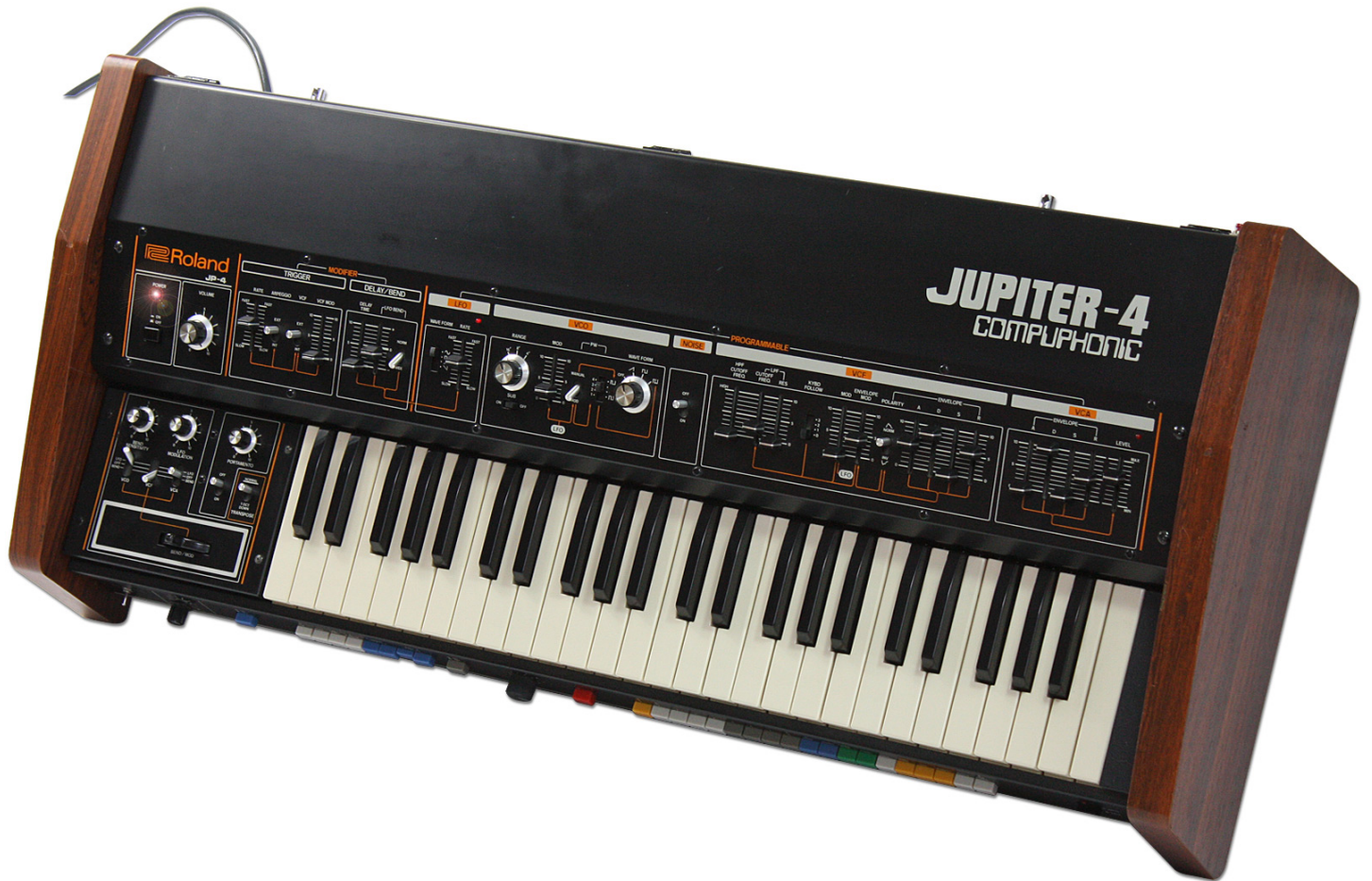
Roland Jupiter-4 with Kenton MIDI and expanded COMPU-MEMORY (8x8 user-memory locations).
