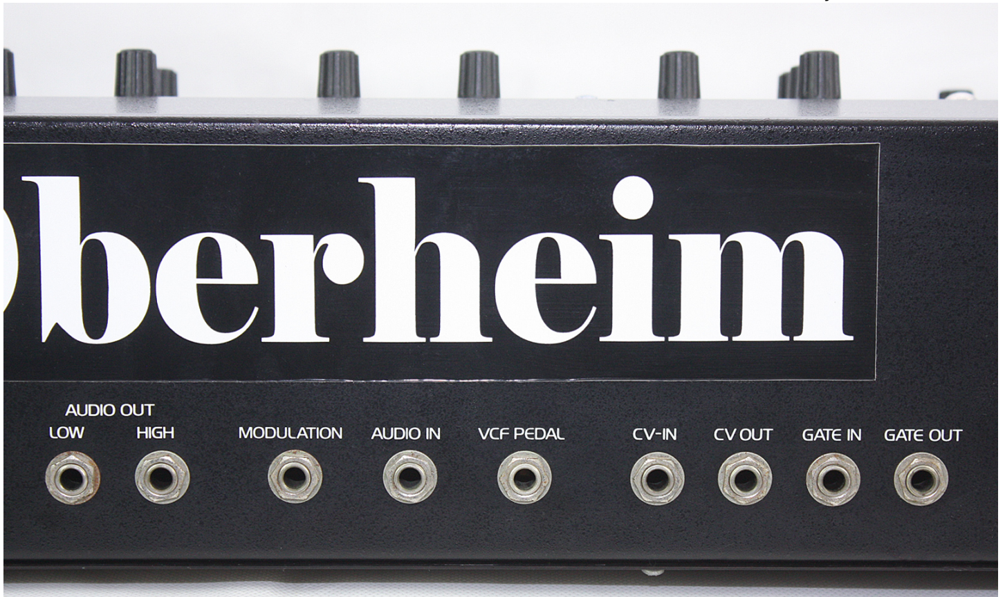
The original OB-1 (black version) has a LOUDNESS input instead of the later OB-1A MODULATION input.
