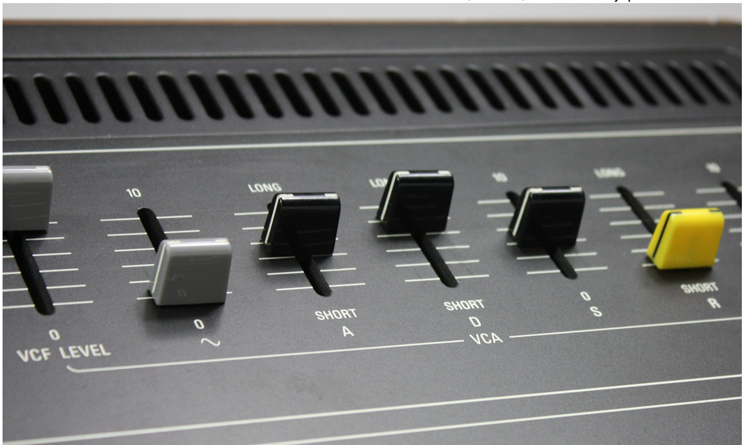
VCA signal-mixer: VCF level and unfiltered sine-wave.
