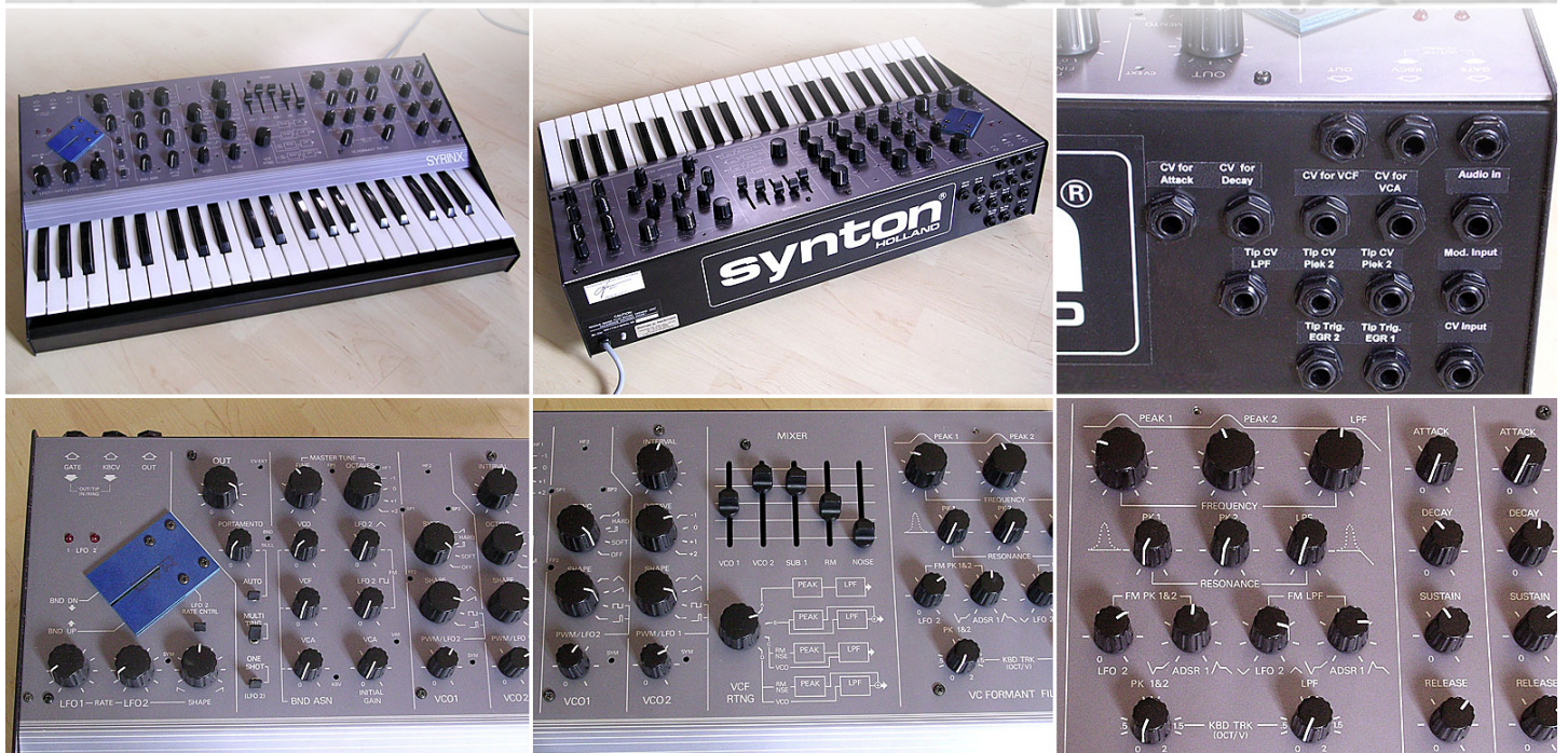
Images of an upgraded Syrinx. According to Peter Forrest, such modifications (patching sockets) were still available in the late 90s.
