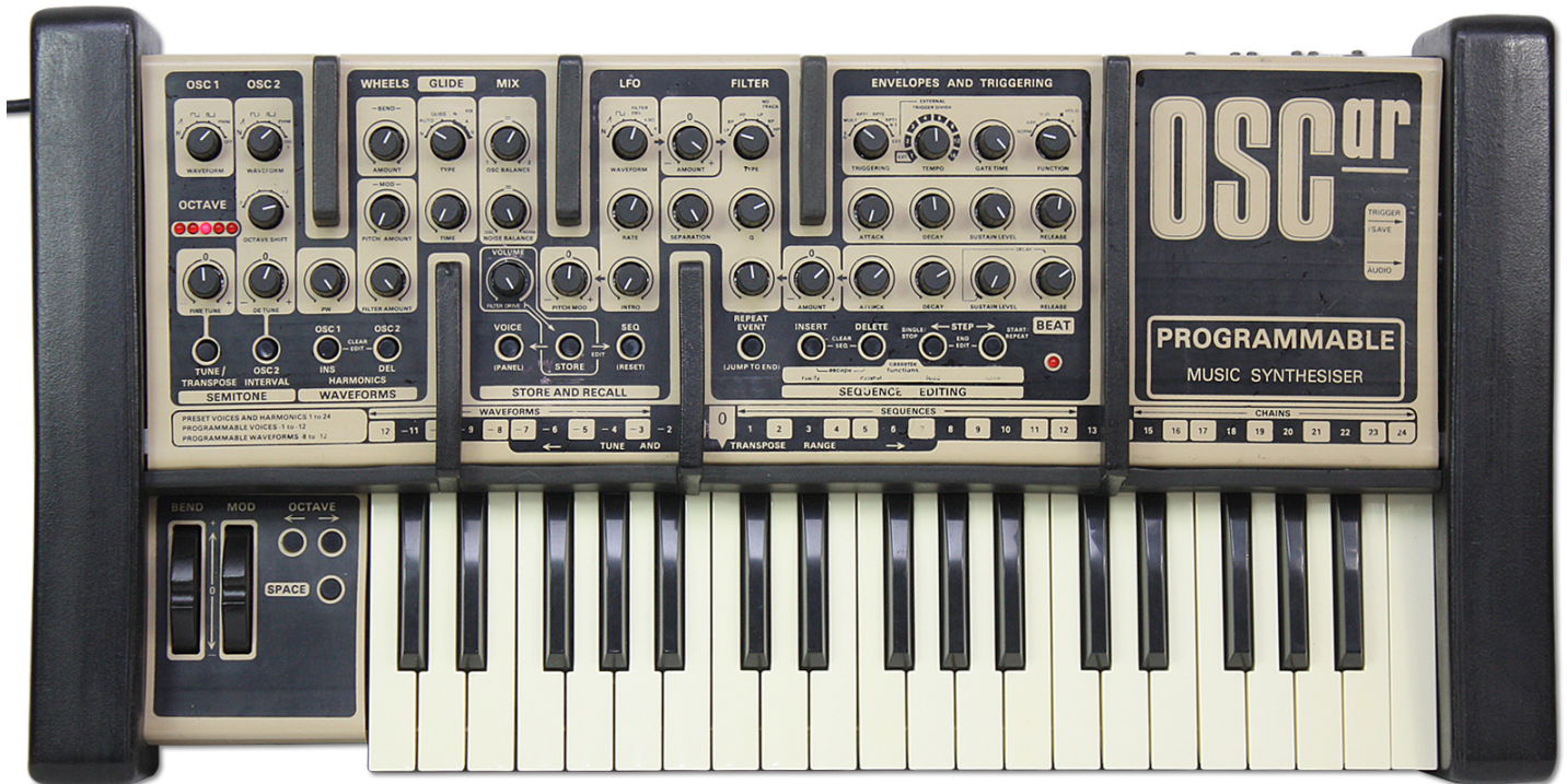
A well-used OSCar with uneven casing, scratches and partially faded lettering. When played, the top C key rubs against the right-hand end-cheek.
