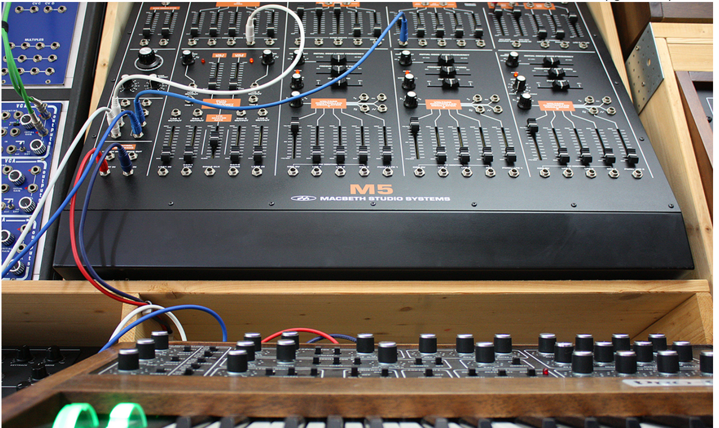
Pro-One serving as masterkeyboard for the MacBeth M5. CV/gate (keyb/sequ/arp) are the red/dark blue cables. Pro-One PitchBend-Out (white) and ModMatrix-Out (light blue) go to VCF2 / VCF1 of the M5.
