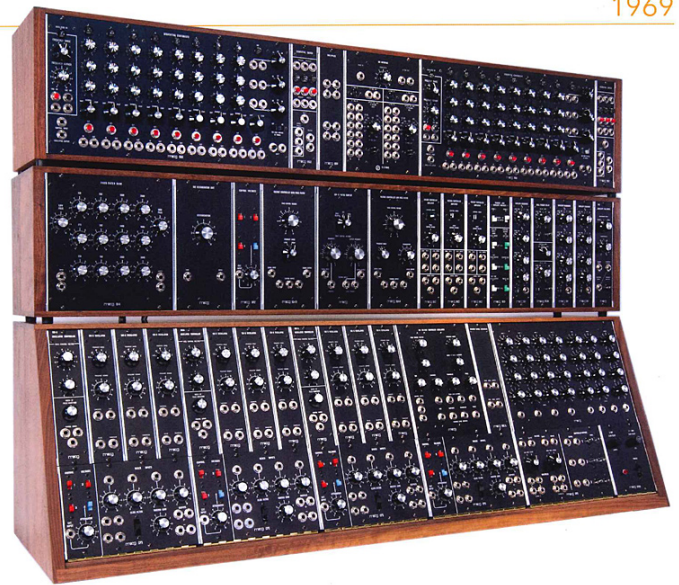
Above: Synthesizer IIIc with Sequencer Complement B on top. Below is the IIIp version of the same configuration.
