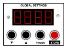
All operations are made with buttons **PROGR**, **STORE** and the couple **INC** (pointing up arrows) and **DEC** (pointing down arrow). Every command has an abbreviated form displayed on the four alfanumeric digits.
